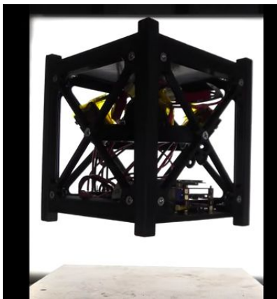
Figure D.4.4-1: Tetrahedral reaction wheel 1U prototype being tested in the PSU Dryden Microgravity Drop Tower. For a video of drop test, please see https://www.youtube.com/watch?v=cC2FpmCP5B4
