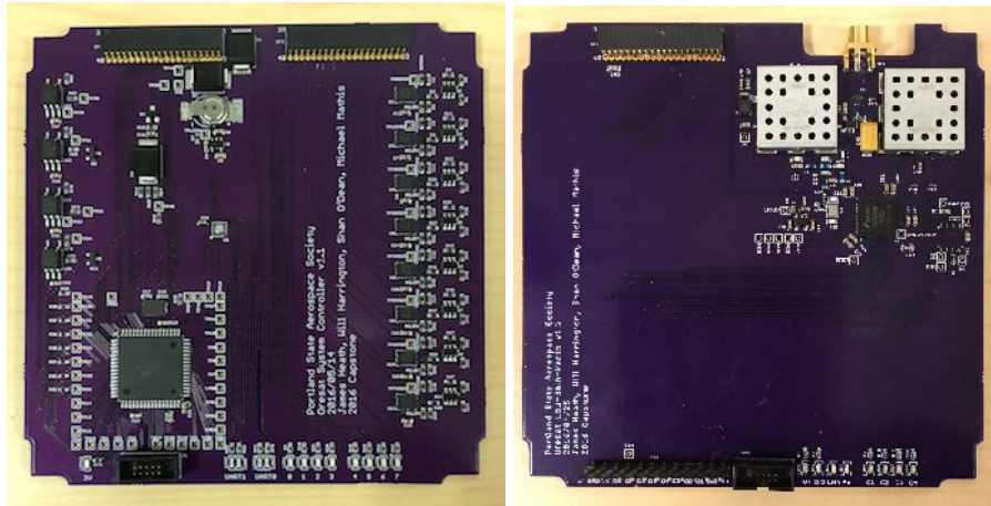
Figure D.3.4-1: Left: OreSat System Controller prototype, with ATmegaS128 Right: Low Gain Radio Board
