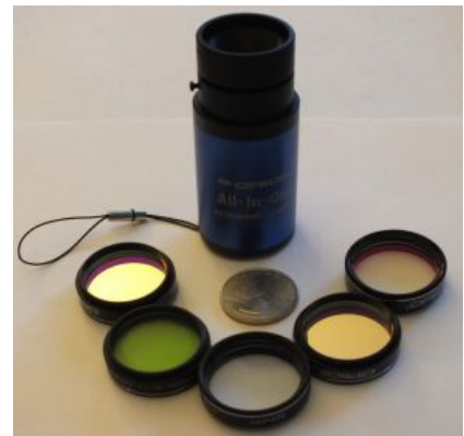
Figure 3: Prototype Astrophotography camera with filters used during ground testing
